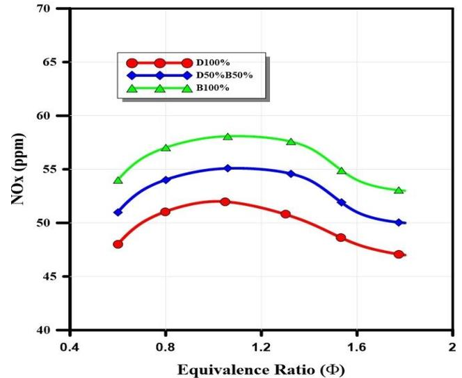
Figure 5. The relationship between NOx emission variation and equivalence ratio.
