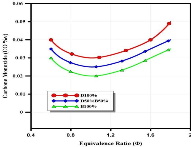
Figure 3. The relationship between CO emission variation and an equivalence ratio.
