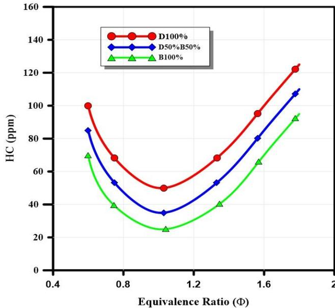
Figure 4. the relationship between HC emission variation and an equivalence ratio.
