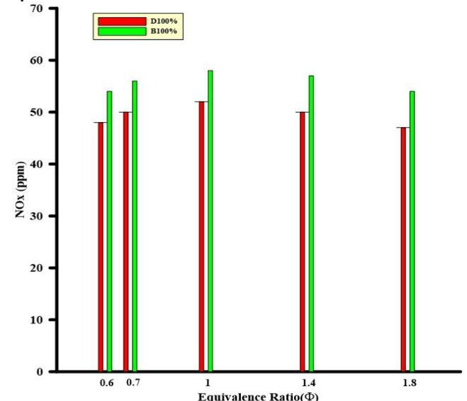
Figure 6. NOx emission of D100% and B100% according to variation of equivalence ratio.
