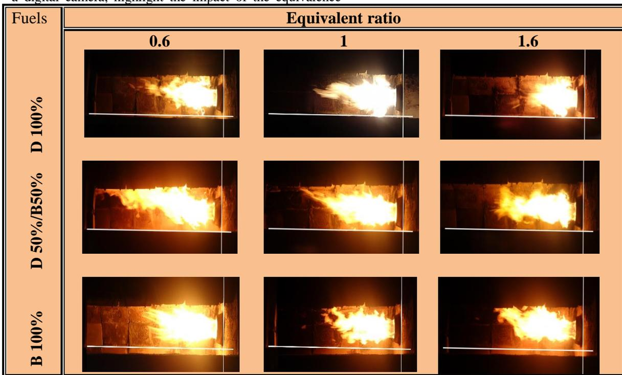
Figure 13. The images of flames of different fuels at various equivalence ratios.
