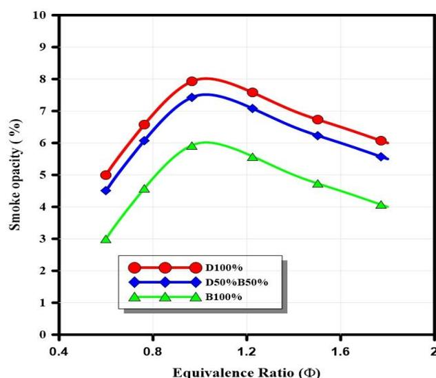
Figure 7. The relationship between the soot emission and equivalence ratio at different type fuels.
