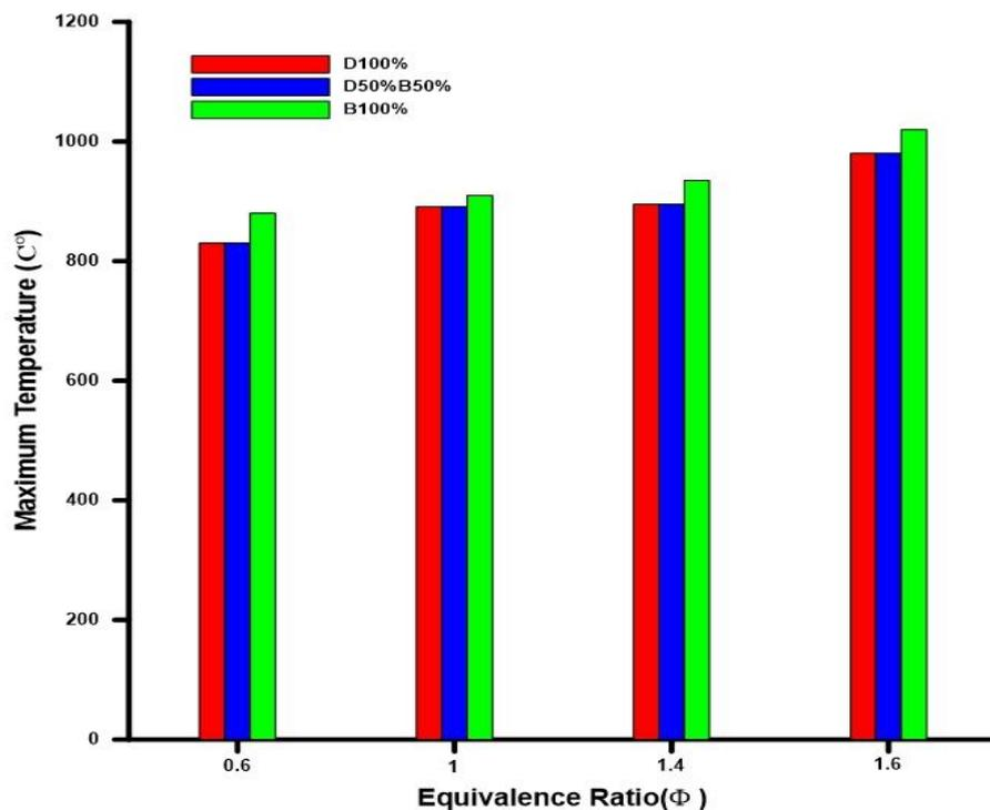
Figure 9. The relationship between change in maximum flame temperature and equivalence ratio
