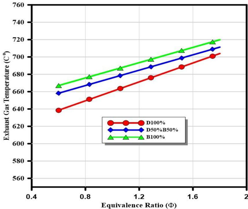
Figure 8. The relationship between change in exhaust gas temperature and equivalence ratio
