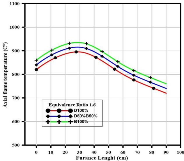
Figure 12. The flame temperature at the centerline of a furnace at an equivalence ratio equal to 1.6.
