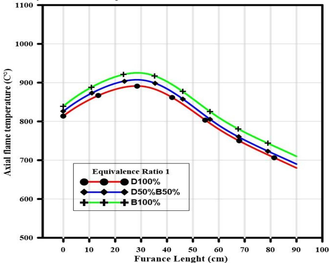
Figure 11. The flame temperature at the centerline of a furnace at an equivalence ratio equal to 0.1.
