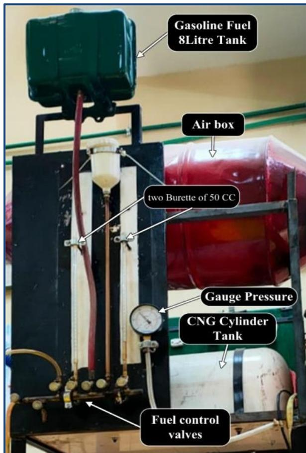
**Fig. 4. Fuel measurement and control system**
