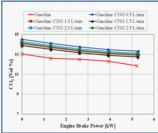
Fig. 9. The fluctuation of CO<sub>2</sub> under different load scenarios
