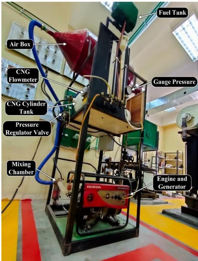
Fig. 2. test rig main view
