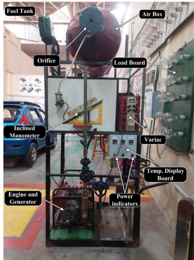
Fig. 3. test rig main view
