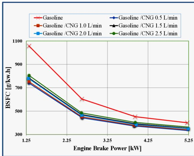
Fig. 6. The fluctuation of BSFC under different load scenarios
