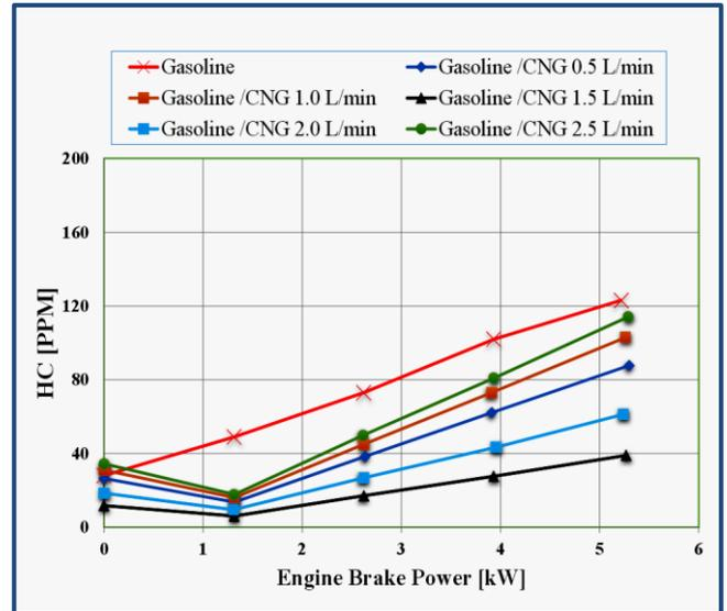
Fig. 11. The fluctuation of HC under different load scenarios
