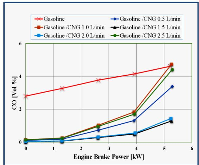
Fig. 8. The fluctuation of CO under different load scenarios
