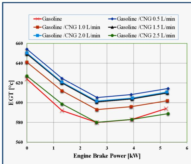
Fig. 7. The fluctuation of EGT under different load scenarios
