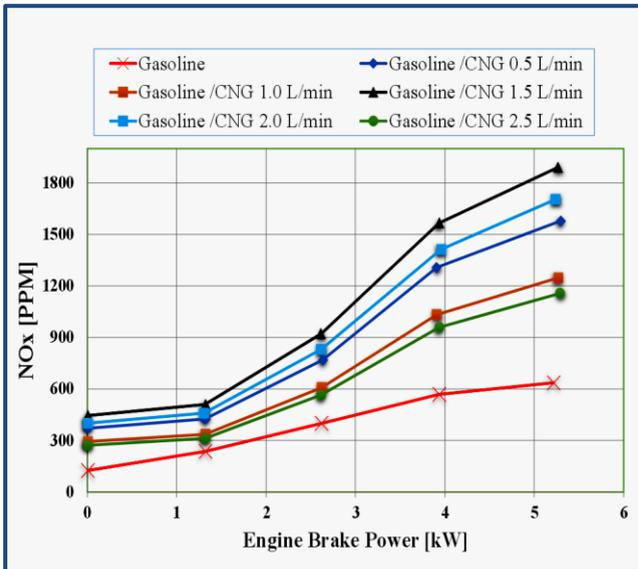
Fig. 10. The fluctuation of NO<sub>x</sub> under different load scenarios
