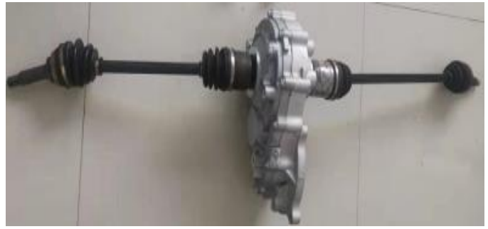
Gearbox + Half shafts: Transfers torque from the electric motor to the wheels, reinforced to handle increased torque loads and minimize power loss while ensuring drivetrain durability.
