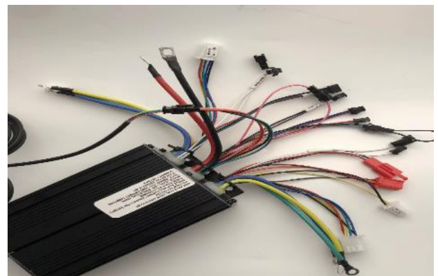
Regenerative motor: Manages bidirectional power flow between motor and battery during acceleration and braking, recovers energy during deceleration, and includes integrated safety features and EMI-shielded wiring.
