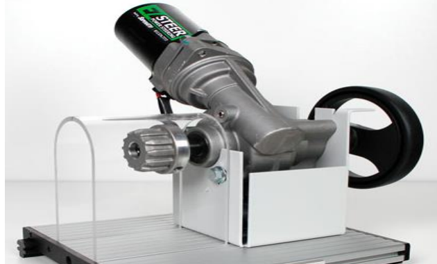
Electric power steering: Replaces hydraulic systems to reduce energy consumption by up to 40%, offering adaptive steering assistance based on vehicle speed for better control and efficiency.
