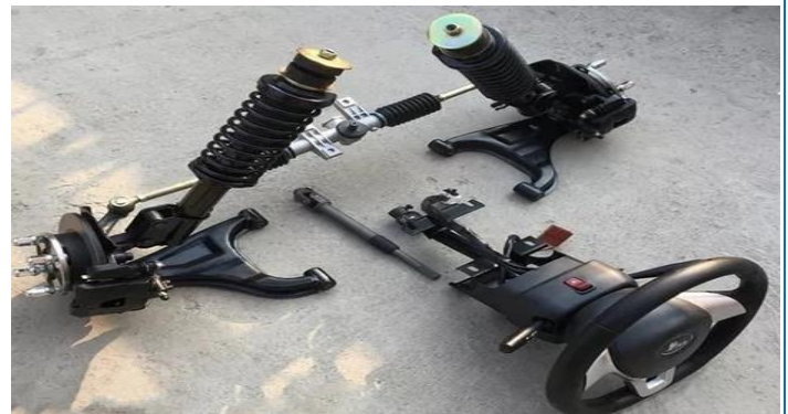
Front steering and suspension kit: Reinforced with upgraded shocks, springs, and arms to handle the added weight of EV components, improving stability, ride comfort, and load handling.
