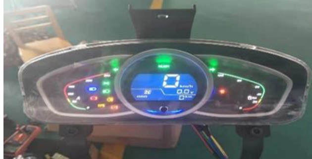
Dashboard 96V: Displays key real-time data such as state of charge, speed, and energy consumption, and includes warning indicators for critical system faults like over current or overheating.
