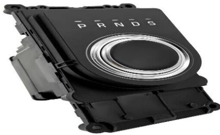
Gear selector: Digitally switches between drive modes (forward, reverse, neutral) without mechanical linkages, simplifying operation and reducing mechanical wear.
