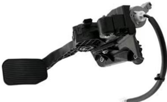
Accelerator: Converts driver pedal input into a 0-5V voltage signal sent to the controller, enabling precise speed and torque regulation with linear response and vibration resistance.
