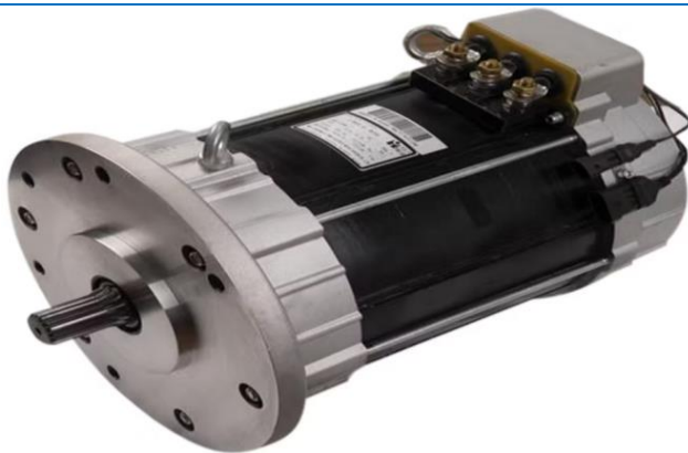
Electric motor 15KW 96V AC: Serves as the main propulsion system by converting electrical energy into mechanical torque (up to 70 Nm) with high efficiency (up to 95%) and minimal maintenance due to its brushless design.
